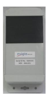
The EVX1150 tag functions both as a wide-area cellular asset tracking tag and a cloud-gateway for the EVX1000 family of robust self-configured IoT asset tracking and wireless sensing networks.
