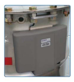
The EV3-ES1 RFID tag is a 433-MHz, active RF device containing a suite of sensors that are powered by long-life batteries, with an omnidirectional read range of ≈100 m. Integrated sensors monitor temperature, humidity, seal integrity and physical shock as well as battery status.
